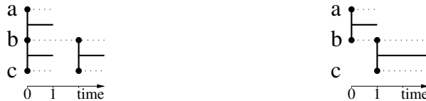
Figure 2: Two stream graphs with n = 2 nodes, m = 1 link, but with different densities: Left: \delta = 0.75 . Right: \delta = 1 .
